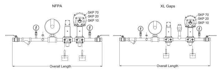
When using the Siemens SKP20 and SKP70 actuators for pressure regulating and ratio regulating functions, the sensing piping is not included. For proper operation, the sensing pipe should be at least 1/4" I.D. and connected a minimum of 5 pipe diameters downstream in a non-turbulent area.
